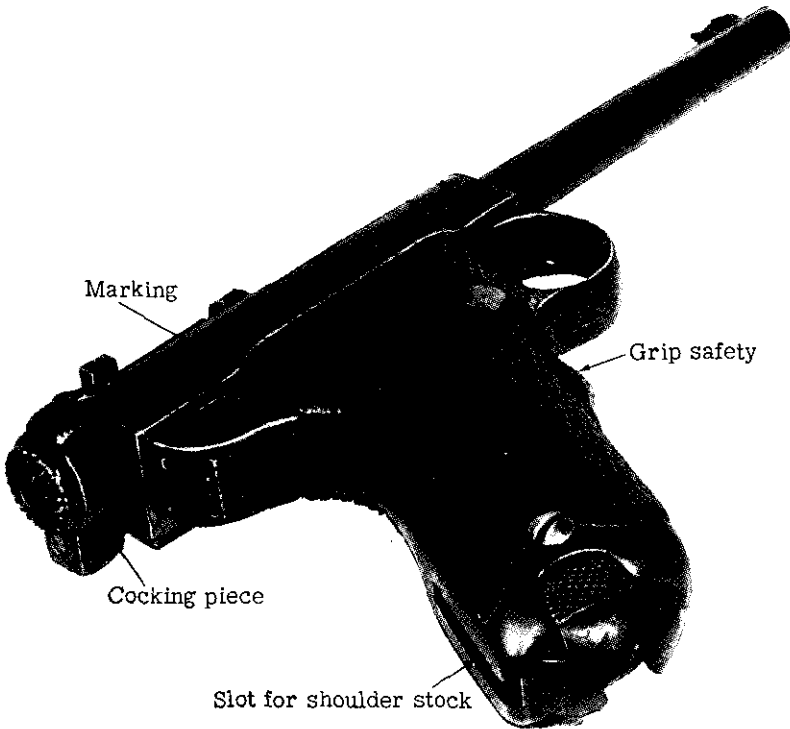
Figure 3.—Nambu 8-mm pistol (three-quarter view), showing marking on right side.
