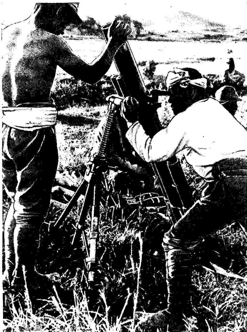
Figure 99.—Laying-in Model 94 (1934) 90-mm mortar.
