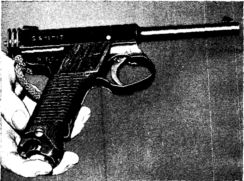
Figure 11.—Model 14 (1925) 8-mm pistol (right side), showing lanyard.
