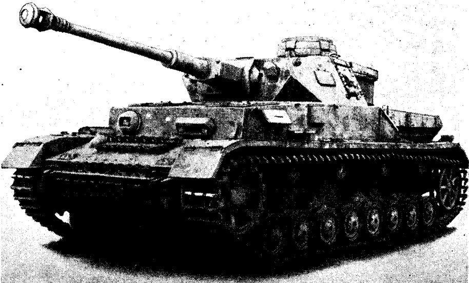
Figure 51.—Pz.Kpfw. IV (with 75-mm long-barreled tank gun). (Weight, 26 tons; maximum speed, 25 miles per hour; armament, one 75-mm short-barreled tank gun (7.5 cm Kw.K.) or one 75-mm long-barreled tank gun (7.5 cm Kw.K. 40), and one 7.92-mm machine gun in turret, and one 7.92-mm machine gun in hull.)
