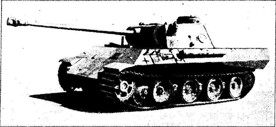
Figure 52.—Pz.Kpfw. Panther. (The present model, which is the newest of the German tanks, has been in action on the Russian front. Weight, 50.5 tons; maximum speed, 30 miles per hour; armament, one 75-mm super-long-barreled tank gun (7.5 cm Kw.K. 43) and one 7.92-mm machine gun in turret.)
