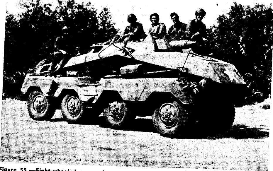
Figure 55.—Eight-wheeled armored car (with 75-mm short-barreled tank gun). (The car has been captured and reconditioned by U.S. troops.)
